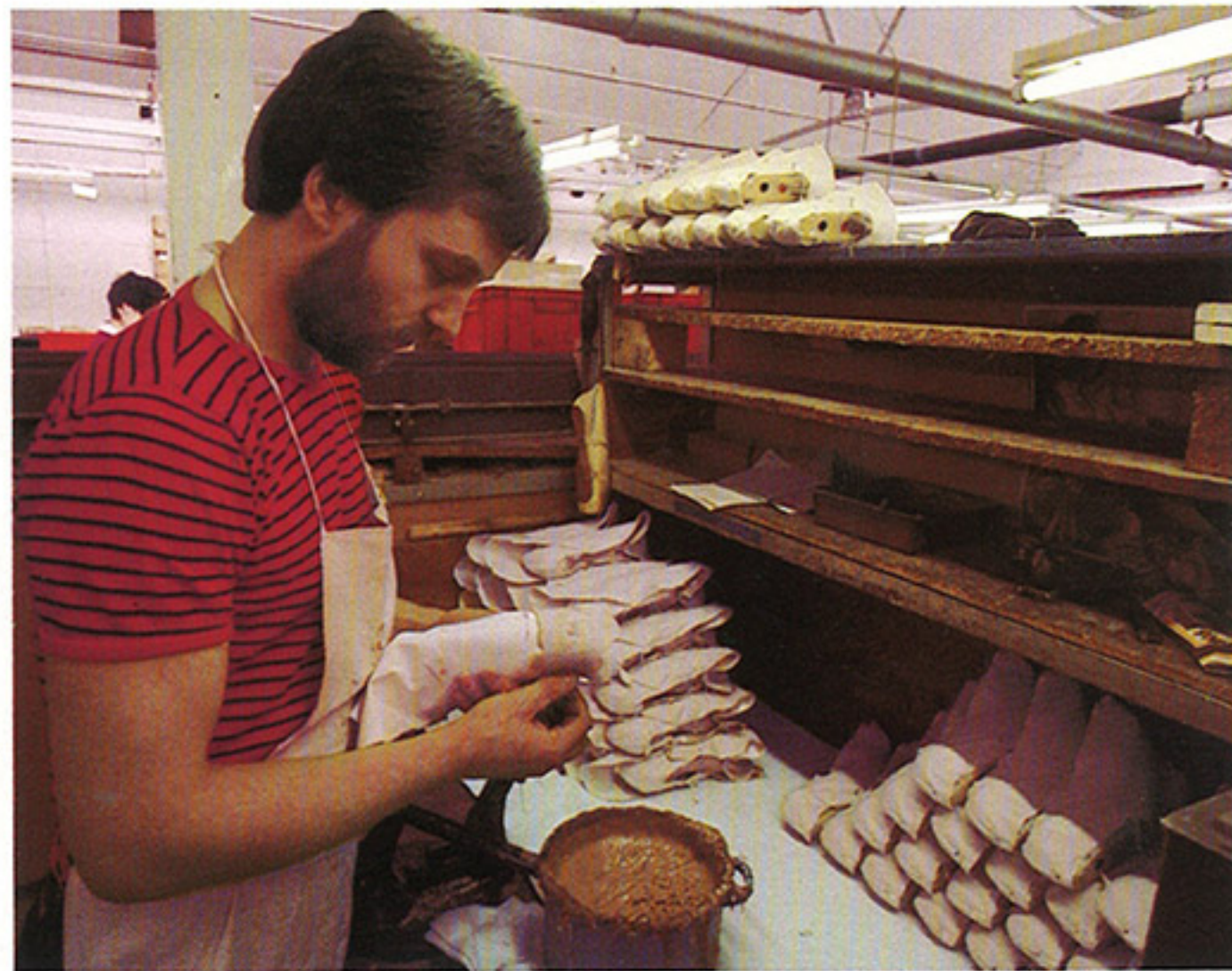
Author's "maker," Ron Boorman, glues layers of satin, paper and burlap to make hard block in toe of shoe.
